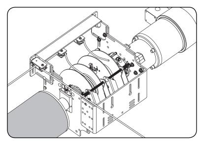
Reattach the bracket tops to the bracket backs with the 3/8-16 x 3-3/4" bolt and 3/8-16 nylock nut. Then, thread the opposite-end return rope through the bracket rope tube to protect the rope from abrasion and sagging. Reattach the rope to the rope reel and run the cover across the pool.
