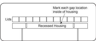
Set one bracket at every gap between the lids. Make sure that 24" is the maximum space between each bracket.
