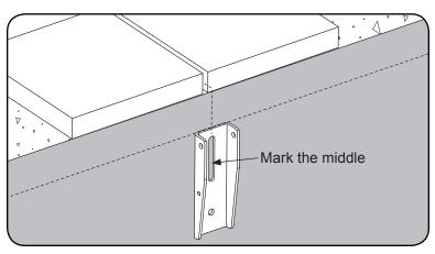
Drill and set an anchor about 1/2" below the middle of the bracket back plate. The anchors must protrude at least 5/8" but less than 1".
