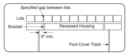
2 Mark the inside of the housing wall at each lid gap.
