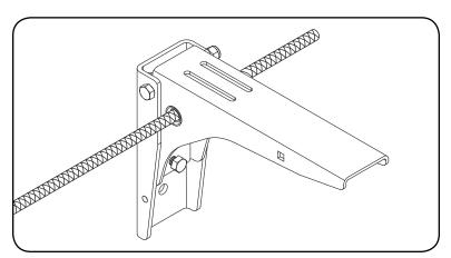
4 Level the bracket top by tightening or loosening the 3/16 x 3/4" bolt. If further adjustment is needed, reverse the bolt so the head of the bolt is against the bracket back.
