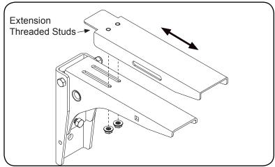
Adjust the bracket back plate up or down as needed. Make sure the plate is level. Mark the remaining two mounting holes. Make sure that the top mounting hole is as close to the top of the bracket as possible.
