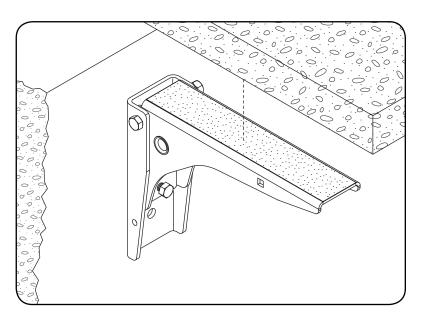
Adjust the lids into position. The edge of the Vanishing Lid should be centered on the top of the bracket. Do not cantilever the lids more than 1/2" on brackets with skid grip; use extensions if the lid extends more than 1/2".
