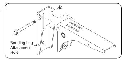
If the bracket uses an extension, set the extension threaded studs into the slots in the bracket top. Adjust the extension to the desired length. Then, attach the extension with two 1/4-20 flange nuts.
